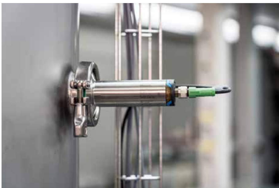
The flush-mounted stainless steel sensor ensures perfect insight into tank condition.
